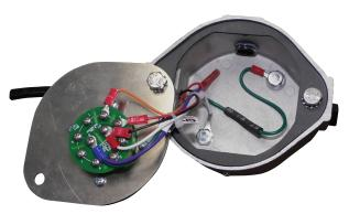
4432-4432 Wiring Shown 4432-4432 Thermistor Socket (Green)
