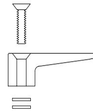
When installing push plate, washers may be necessary to achieve proper operation of interlock. (P/N 301)
